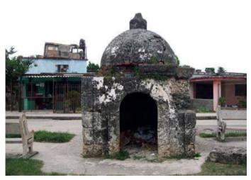
**Fig. 5**. One of the small towers that protected the ventilators of Fernando VII aqueduct in Independence street.
